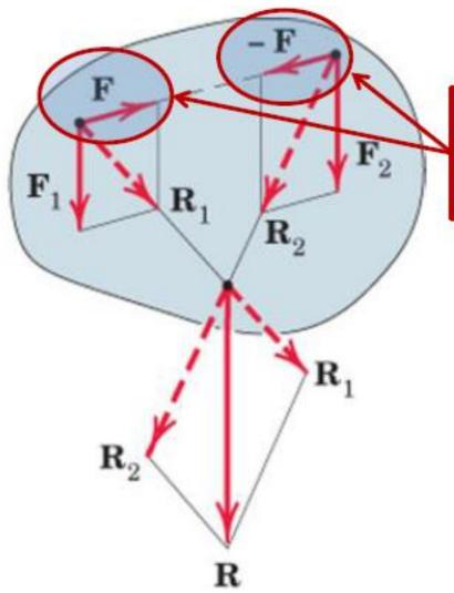
Adding two opposing forces F and –F with the same line of action will not alter the mechanics of the body
